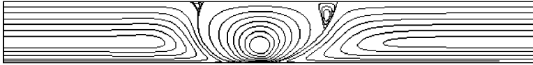
FIGURE 8. The streamlines for the flow field from the FEMLUB model using a silicone-oil drop and air with d = 0.93 , Re = 23.756 , and q = 0.00256 . This is not a converged steady solution.
